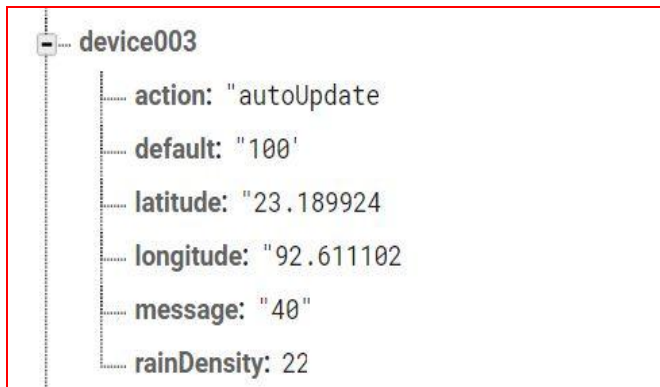
Figure 5. Data format of the status of a device in database
